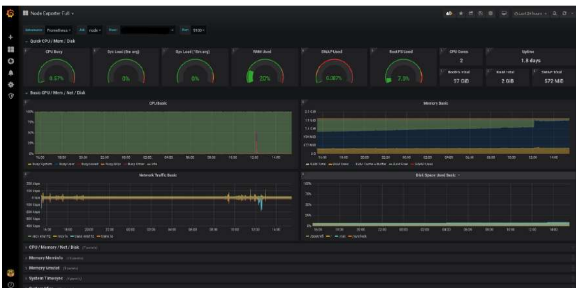
Figure 1: Grafana displaying a Dashboard of metrics from Node Exporter (Node Exporter Full, 2022)
